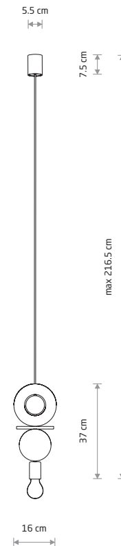
DROPS WOOD E plywood, painted steel
